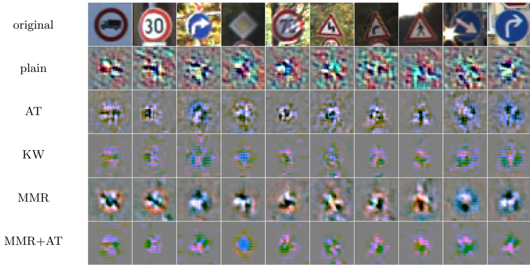
Figure 3.8: Gradient of l_\infty -robust models. We visualize the gradients of the cross entropy loss wrt the input for different images of GTS test set (first row) for every model: plain training, adversarial training [Madry et al., 2018], KW robust training of Wong and Kolter [2018], MMR, MMR + adversarial training. We can see for robust models the gradients are much sparser, while only for plain training it does not clearly highlights relevant features.
