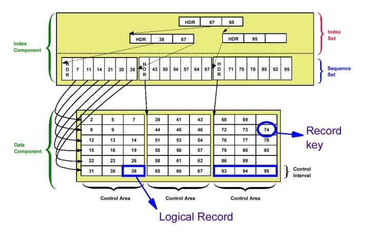
VSAM stands for Virtual Storage Access Method. It is a method of managing files that is used mainly on mainframes. Specifically, VSAM can speed up access to file data by using a reverse index of records appended to files.
