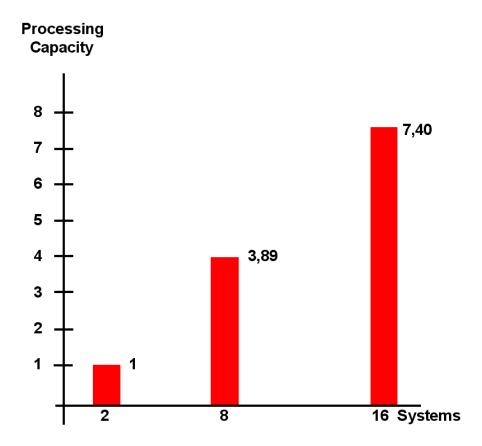
The above graph shows Parallel Sysplex performance degredation. It has been copied from [49]. The benchmark used includes a real life mixture of on-line transaction processing, reservation systems, data warehousing, and banking applications.
