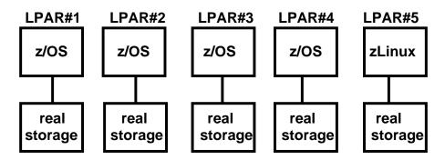
This looks like shown above. LPARs are the equivalent of a separate mainframe for most practical purposes. Each LPAR contains its own operating system and maps its virtual storage into its own real storage. A Hypervisor named PR/SM controls the LPARs.
