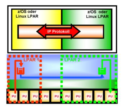
Internal Queued Direct I/O and Hipersockets permit high speed communication between LPARs. It is possible to configure up to 16 internal (virtual) Ethernets within a single mainframe system [41]. This permits LPARs to communicate with each other over what looks like a socket/TCP/IP/Ethernet connection with each other, which in reality is implemented with code and queues in the Hardware System Area.
