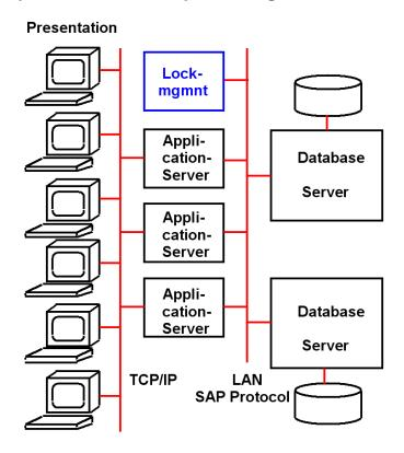
Using a typical SAP R/3 ERP configuration as an example, a group of application servers is supported by an additional Lock management server (Sperr-Server or Enqueue Server in SAP terminology). Whenever an application server wants to acquire or change a lock, it interrogates the lock server as to the lock status.
