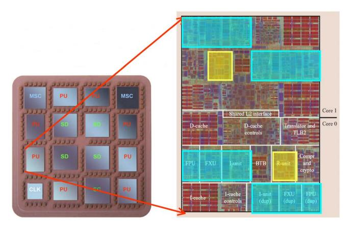
The dual core z9 CPU Chip shown above duplicates the Instrunction unit (I-unit) and both the fixed point (FXU) and floatig point (FPU) execution units to improve error detection and error recovery. This provides a mechanism by which the mirrored execution used for error detection occurs 1 cycle delayed from actual operation, and allows the operation execution logic and circuitry to be optimized for performance [09].
