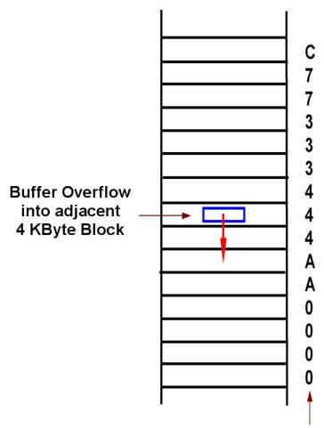
A Buffer overflow into an adjacent 4 KByte block can only occur, if this block happens to have the same storage protection key assigned. A buffer overflow from a user program into a supervisor area is essentially impossible.
