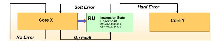
The fully architected state of each processor is buffered in the Recovery Unit (R Unit) on each chip. The RU stores a complete ECC protected copy of the processor state. This includes all registers, independent if they are part of the architecture or not. It collects all error messages and supervises recovery actions for nearly all hardware errors [10].
