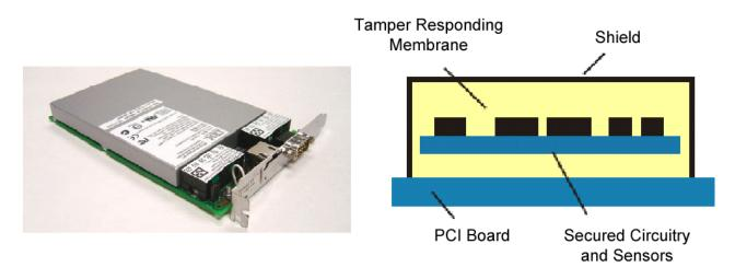
The Crypto Express 2 (CEX2) card uses a Tamper Resistant Security Module (TSRM). Tamper proof crypto cards are an integrated part of System z.
