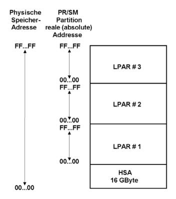
For practical reasons, the real storage of all LPARs is mapped into a single physical storage. Each LPAR is assigned a part of physical storage, using address relocation, with a starting address of hex 00..00. The size of real storage assigned to each LPAR is defined by a system initialization parameter, and may differ between LPARS.
