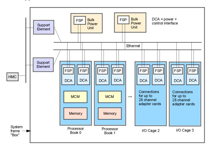
The Support Element (SE) is the central point of control in each Mainframe system. In todays z9 and z10 systems, the SE is implemented by a Think Pad lap top. It is permanently mounted into the mainframe box, and cannot be removed.
