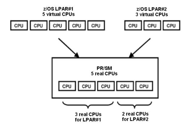
In this example you may assign a weight of 3 to LPAR#1 and a weight of 2 to LPAR#2. This means, LPAR#1 is assured a minimum capacity of 3 CPUs, and LPAR#2 a minimum capacity of 2 CPUs.
