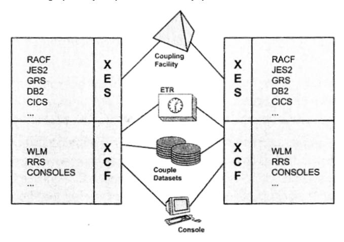
A Geographically Dispersed Parallel Sysplex (GDPS) is an extension of a Parallel Sysplex of mainframes, supporting multiple site configurations, located potentially in different cities. GDPS helps automate recovery procedures for planned and unplanned outages to provide near-continuous availability and disaster recovery capability. Assume for example two sites, one for production, and the other for disaster recovery.
