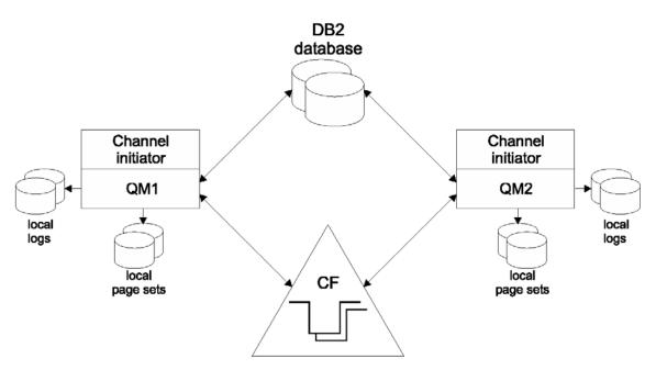
In a Message Based Queuing Application an MQSeries message is sent to a sysplex. Each system in the sysplex contains a Queue Manager (QM) and associated Channel Initiator, able to receive an MQmessage. The group of queue managers that can access the same shared queues is called a queue-sharing group. The Queue Managers are running on separate systems. Each member of the queue-sharing group has access to the same set of shared queues. A coupling facility list structure manages the queues.
