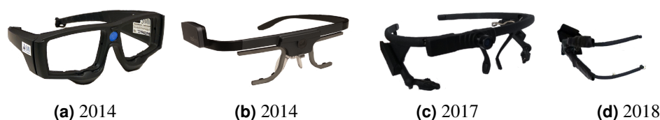
Figure 1.1: State-of-the-art head-mounted eye-tracking hardware evolution. SMI ETG2 (1.1a) and Tobii Glasses Pro 2 (1.1b): cannot be used with glasses. Pupil (1.1c): fitting over glasses is cumbersome and sometimes even impossible. Inconspicuous and modular eye tracker proposed by Eivazi et al. [25] (1.1d): these modules can easily be attached to any glasses or 3D-printed frames [26].
