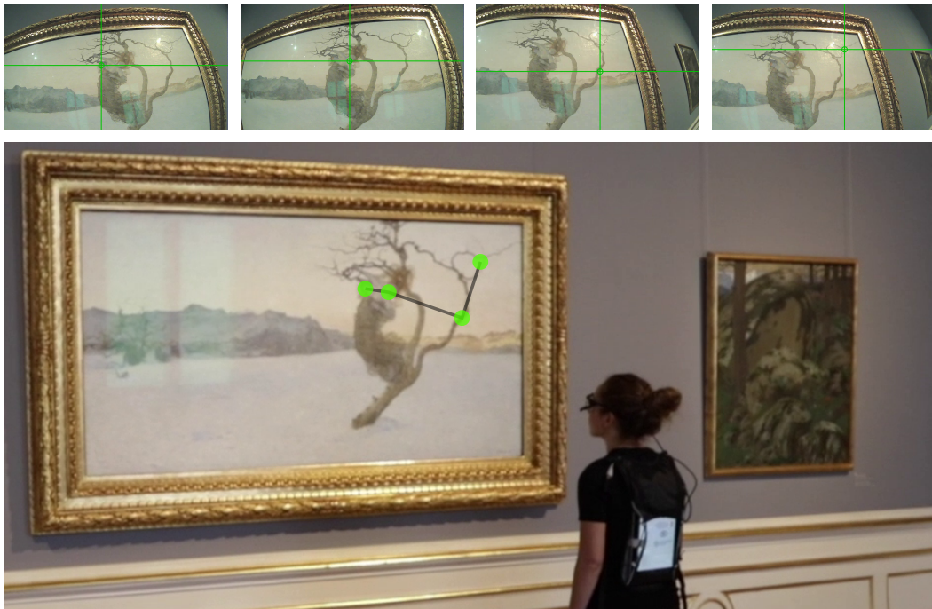
Figure 7.1: Eye-tracking enabled insights. Eye tracking reveals the trajectory of fixations (i.e., the scanpath ) as the visitor attends to Giovanni Segantini’s The Evil Mothers . These scanpaths provide key insights into the human cognitive process and are also useful for distinguishing a subject’s expertise level [291]. Figure best visualized in digital form [53].
