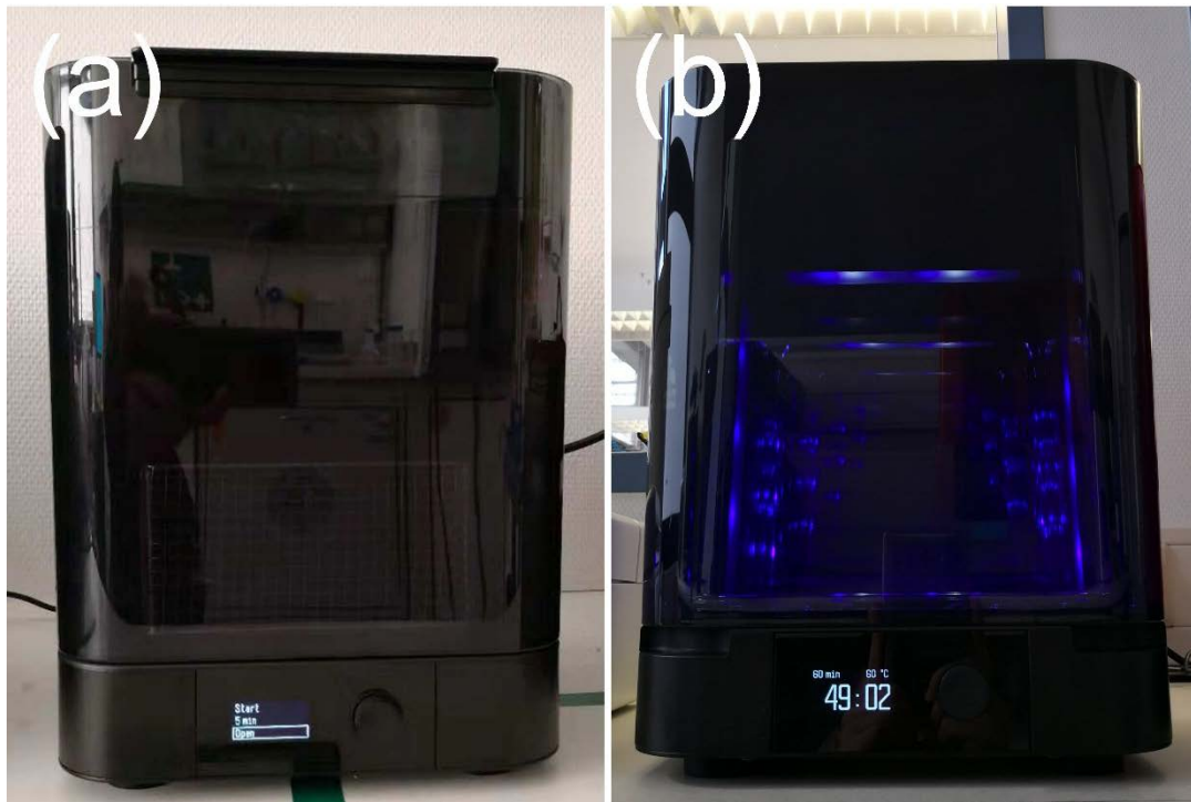
Figure 11: Post-processing devices of the SLA 3D printer. (a) Post-cleaning device “Form Wash”; (b) Post-curing device “Form Cure”.
