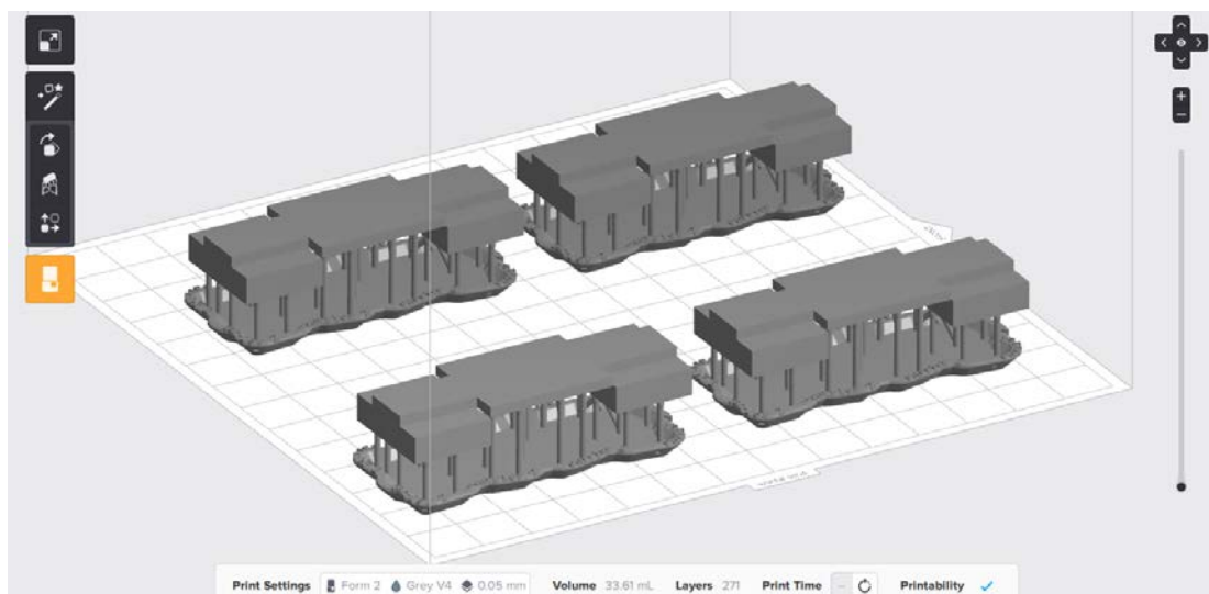
Figure 30: The printing direction and layout of the carrier.
