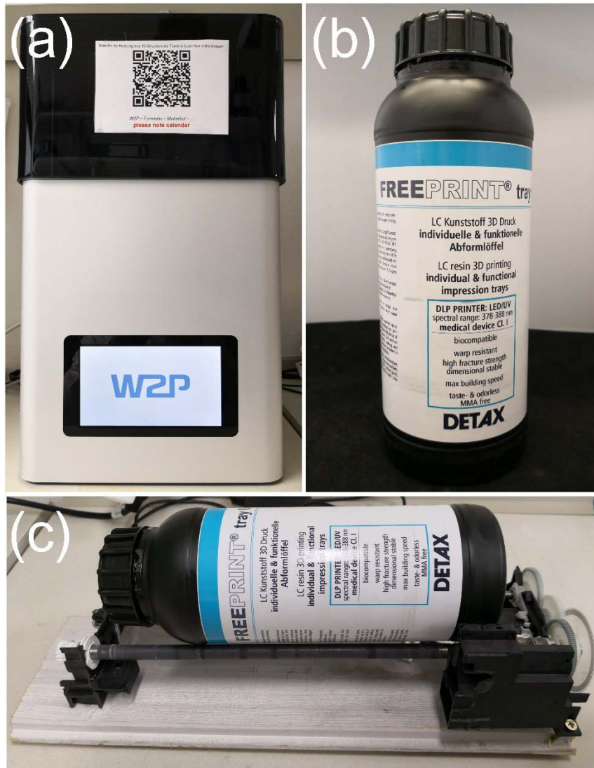
Figure 15: The DPL 3D printer, printing material, and self-developed roller mixer. (a) The DLP 3D printer “SOLFLEX 170”; (b) The custom tray material “FREEPRINT tray”; (c) The self-developed roller mixer.
